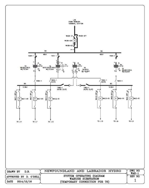
Figure A1: Existing Wabush Substation Single-Line Diagram
