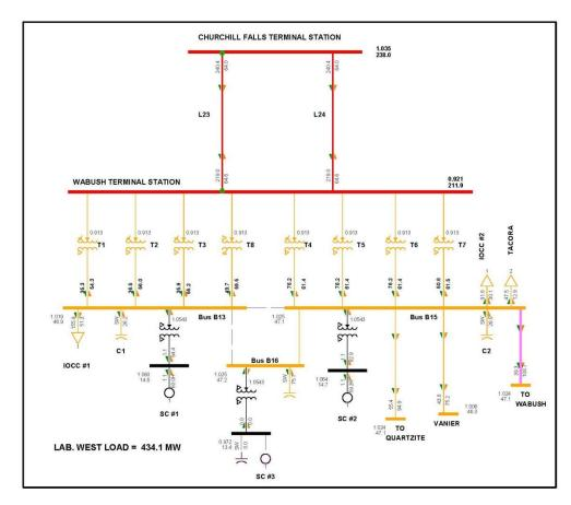
Figure A7: Alternative 5 – 2043 Peak Load Loss of SC3
