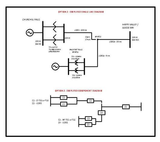
Figure A2: Option 2 – Simplified Single-Line/Component Diagram
