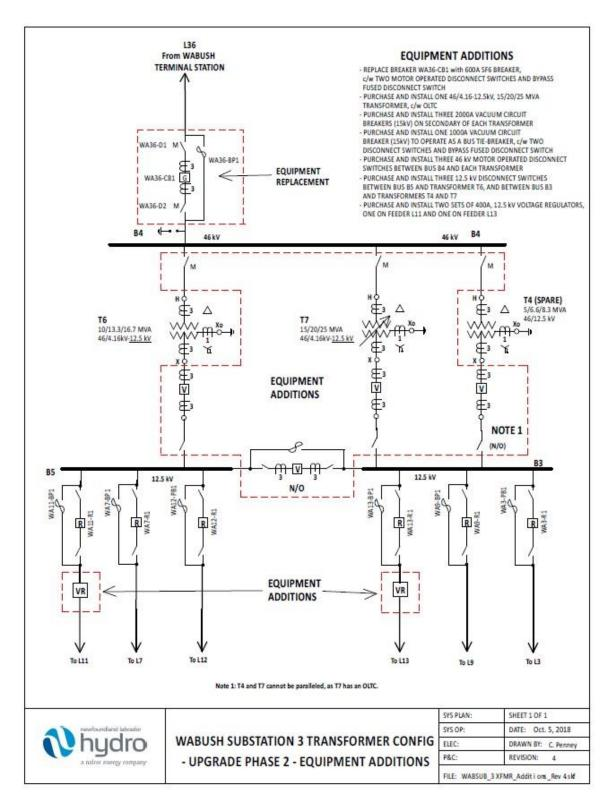
Figure B4: Wabush Substation 3 Transformer Configuration – Upgrade Phase 2 – Equipment Additions
