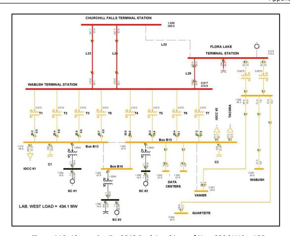
Figure A10: Alternative 7 - 2043 Peak Load Loss of New 230 kV Line L25
