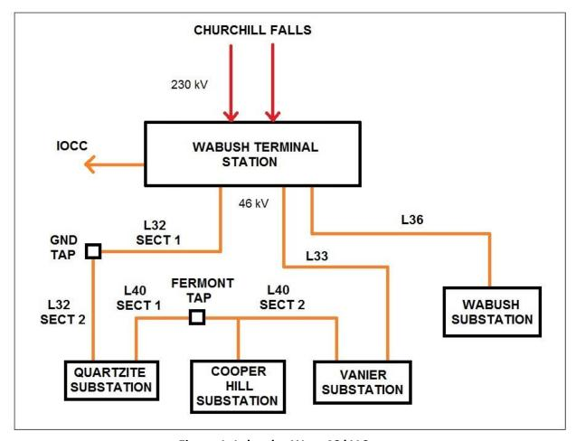
Figure 1: Labrador West 46 kV System
