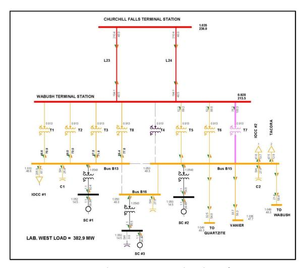
Figure A3: Alternative 4 – 2043 Peak Load Loss of T4
