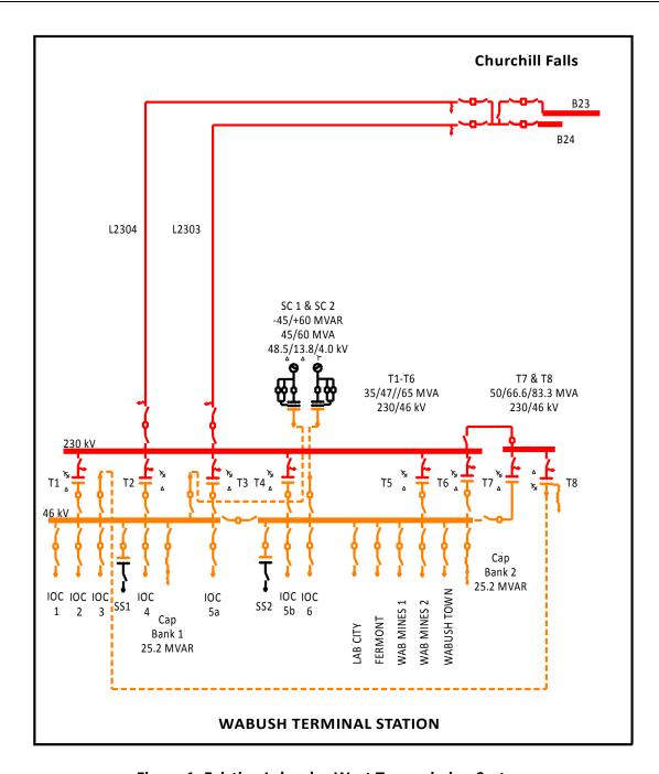
Figure 1: Existing Labrador West Transmission System
