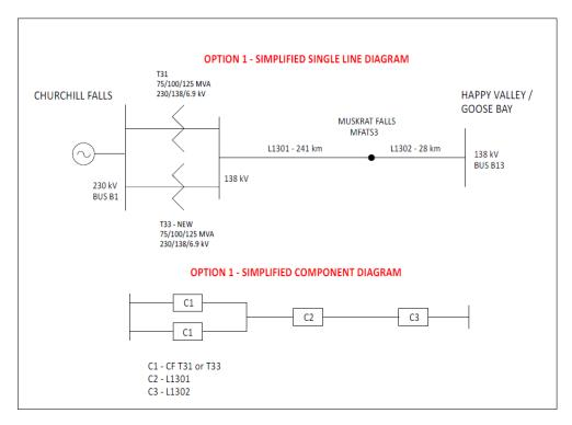
Figure A1: Option 1 – Simplified Single-Line/Component Diagram
