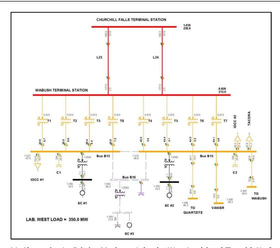
Figure A1: Alternative 1 – Existing Maximum Labrador West Load Capability with No Outages
