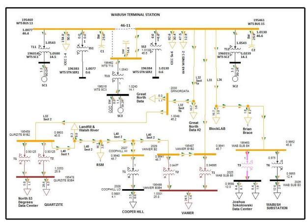
1 A load flow plot of this scenario is provided in Figure A3, below.
