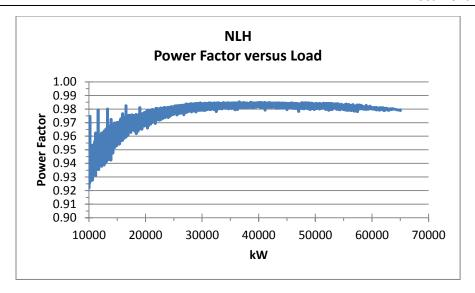
Figure 2: Hydro Power Factor versus Load
