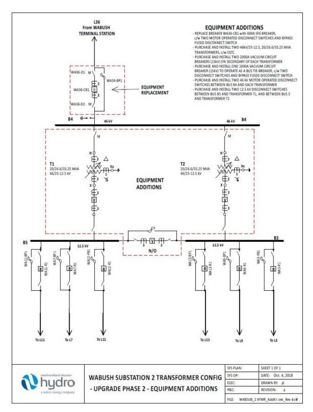
Figure B2: Wabush Substation 2 Transformer Configuration – Upgrade Phase 2 – Equipment Additions
