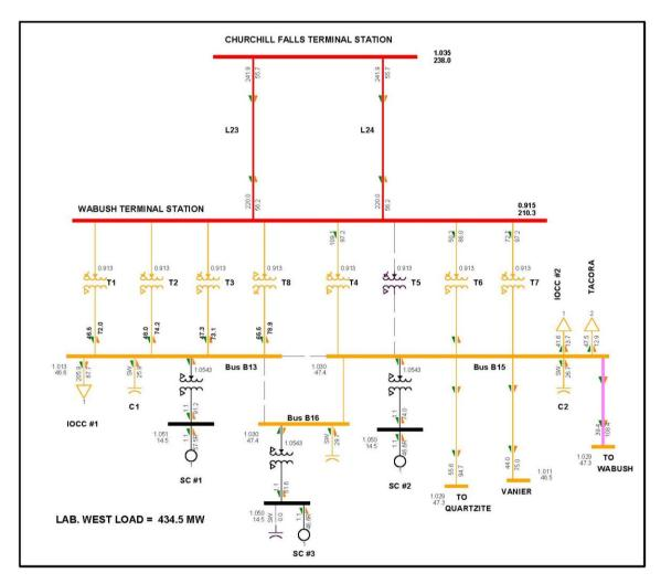
Figure A6: Alternative 5 – 2043 Peak Load Loss of T5
