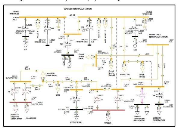
Figure A4: Flora Lake Terminal Station 46 kV – with Data Centres
